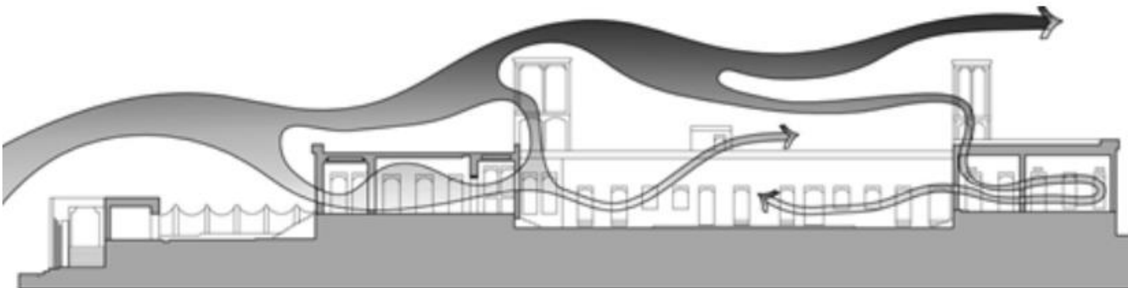
Fig. 1. Airflow System in the Fekri House, Bandar-e Lengeh*
